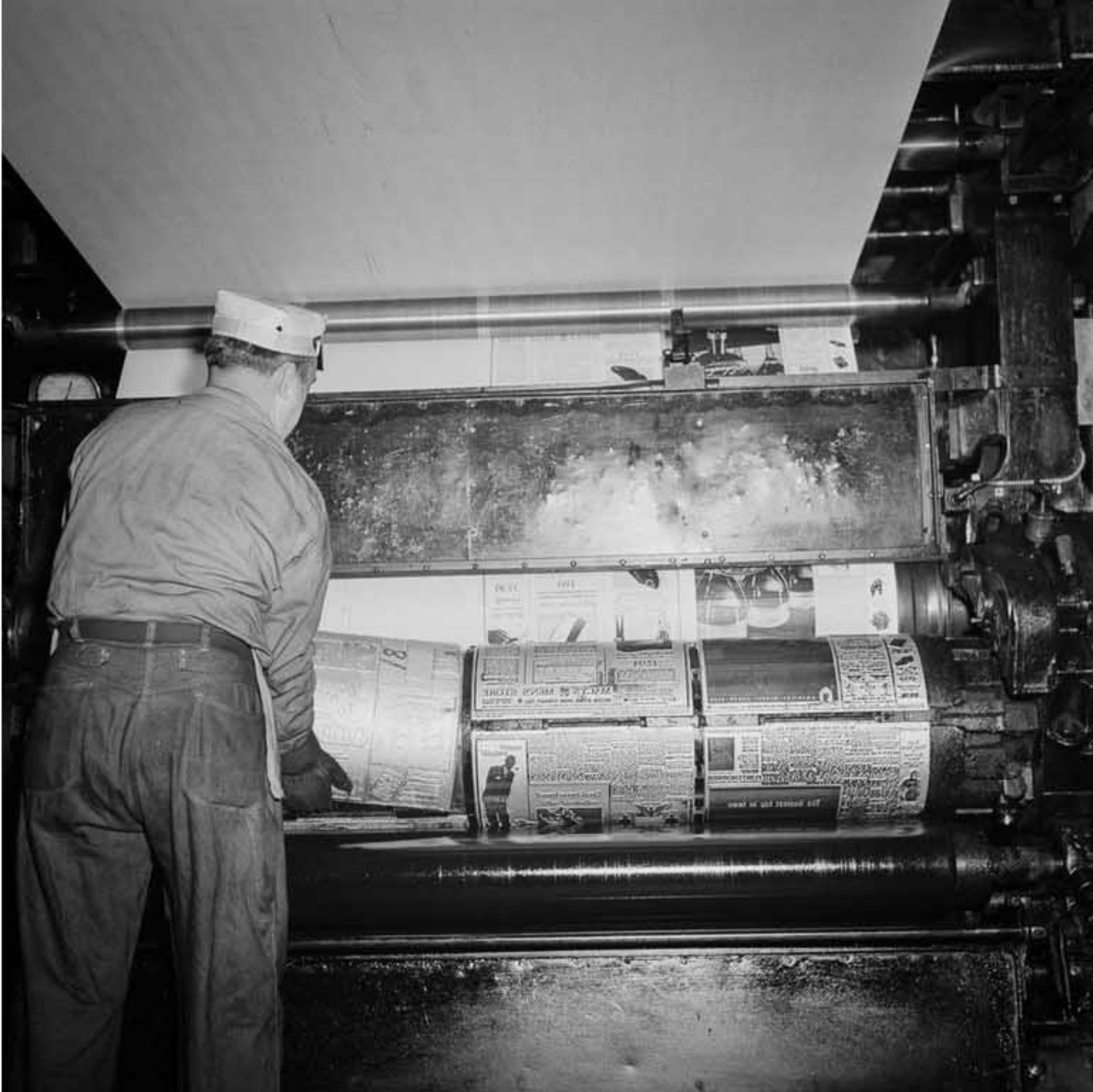
Rotary presses, cont'd: curved stereotyped plates in a rotary press in the New York Times' pressroom, 1942
