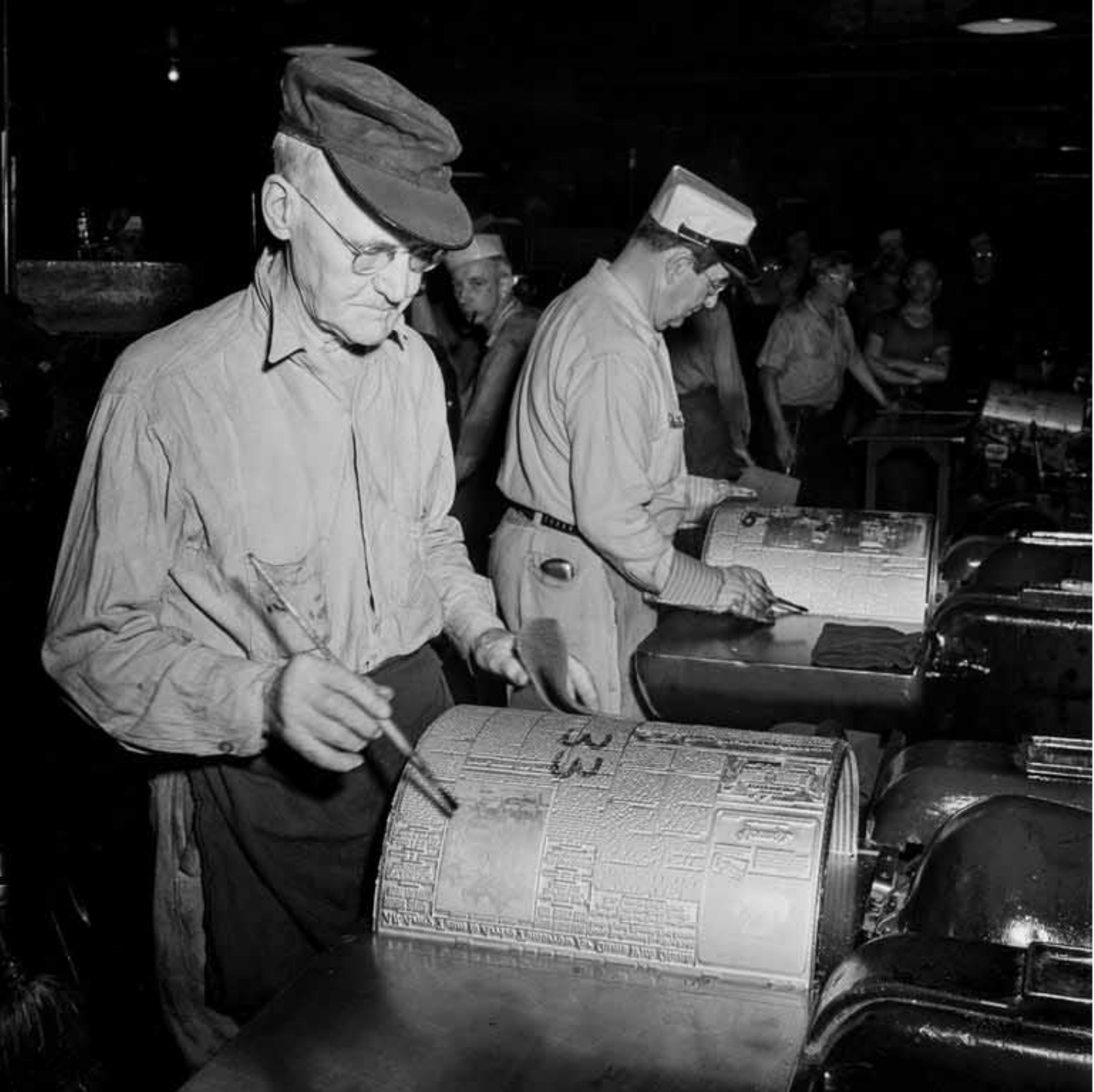
Rotary presses, cont'd: curved stereotyped plates in a rotary press in the New York Times' pressroom, 1942
